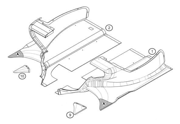
Superficial repairs applied to the removable front floor extensions (n.9&10) are tolerated.
